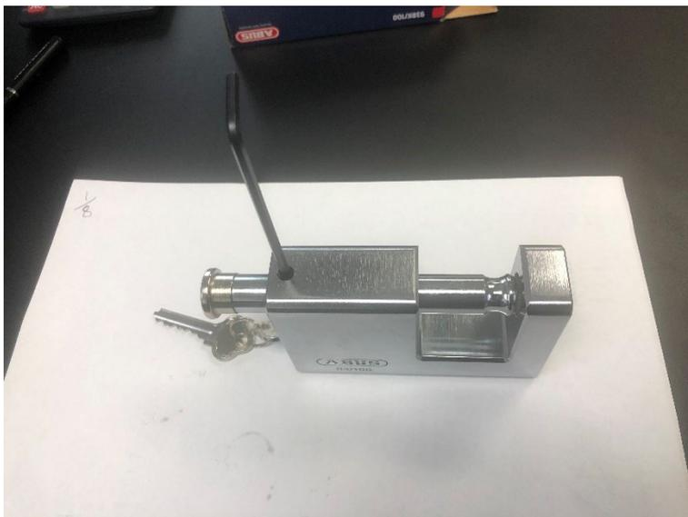
Using 1/8 hex key remove grub screw.
