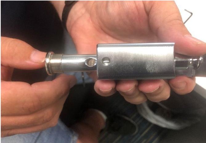
Rotate bolt so both access holes line up.
