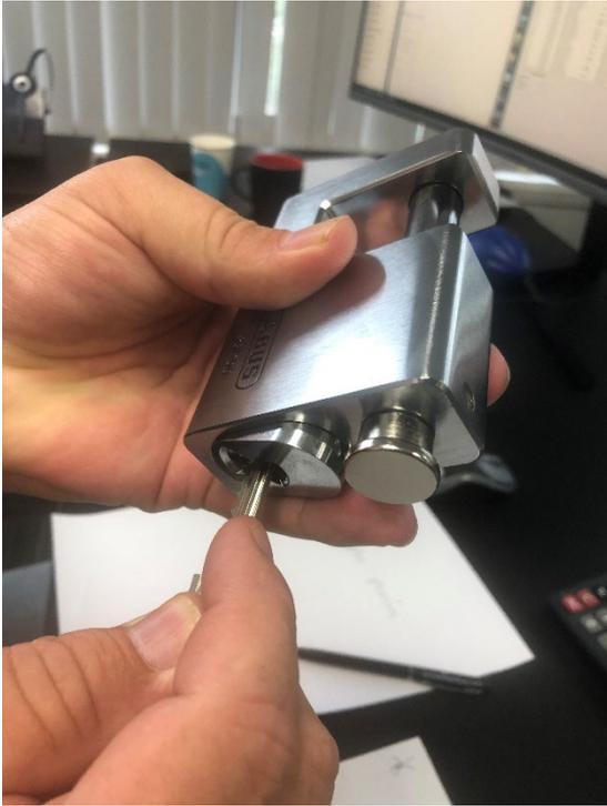
Remove key from cylinder. With padlock keyway facing down press onto cylinder to remove shroud.
